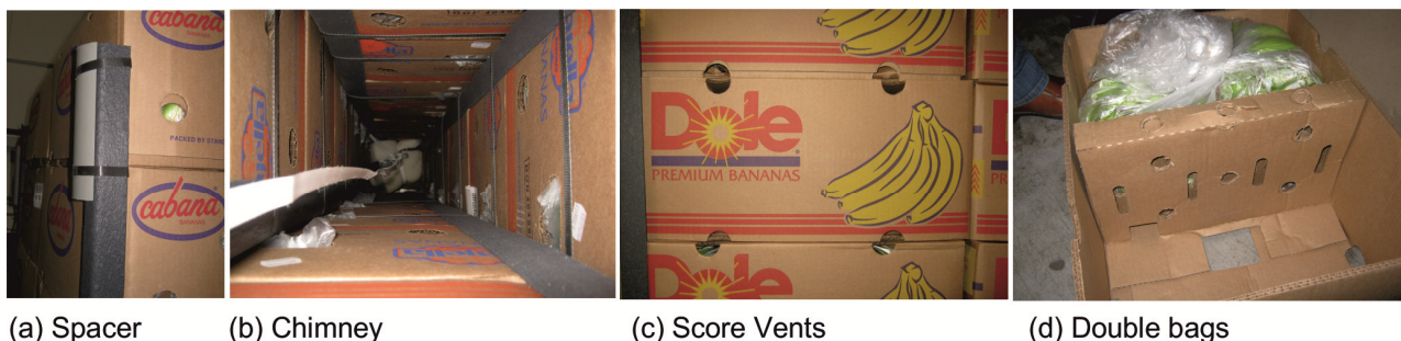
Figure 11. Modifications in packaging and stowage. (b) shows chimney after removing foam block.
