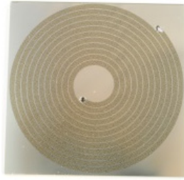
Figure 8: Using the technology of microfluidics, a small GC-column is made for the \mu CG (Sklorz, 2012).
