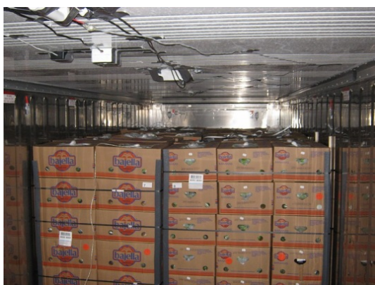
Figure 6: Pallets in test container with antennas for wireless sensors under the roof.
