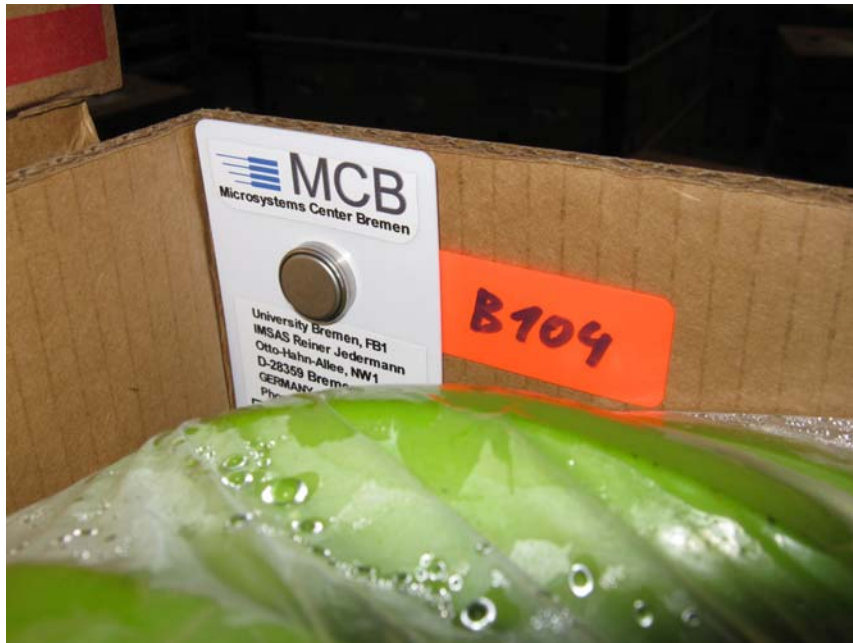
Figure 5: Position of the sensor in the corner of a box. The measured temperature is influenced by supply air temperature, heat transfer through the cardboard box and warming of the supply air at the surface of the bananas.
