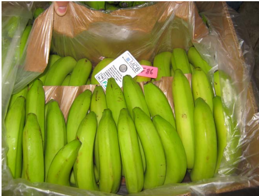
Figure 2: Positioning the iButton temperature loggers between the bananas approximately at the center of the banana box. The plastic film was opened to install the temperature logger.
